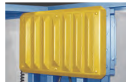
Conditioning plates are offered in standard and custom profiles matched to specific materials and bag designs.
