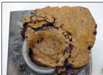
FIGURE 1. After completion of a test, in which self-heating of the product took place, the product was completely burnt. The charred and partly molten remains no longer fit inside the sample holder
