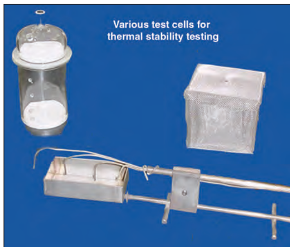
FIGURE 4. (Top left) In the test for “aerated” conditions, air flows through the sample from top to bottom, which are both closed by sintered glass discs. The cylindrical section has a 50 mm dia. and a height of 80 mm. (Bottom) For “air over layer” testing, warm air flows over the powder layer in the sample tray. (Top right) The wire basket for “basket testing” is illustrated more clearly in Figure 5
