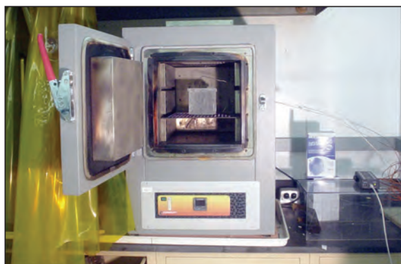
FIGURE 6. This “basket test” sample holder is prepared for testing inside a laboratory oven
