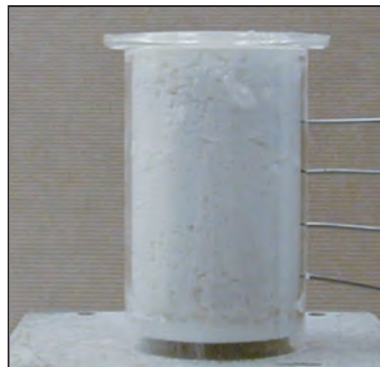
FIGURE 3. In this typical test cell for “bulk” conditions (50-mm dia., 80-mm height), air can diffuse into the sample through the open top of the cell and through the bottom of the cell, which is closed with a sintered glass disc. The sample temperature is measured continuously at various locations along the height of the cell
