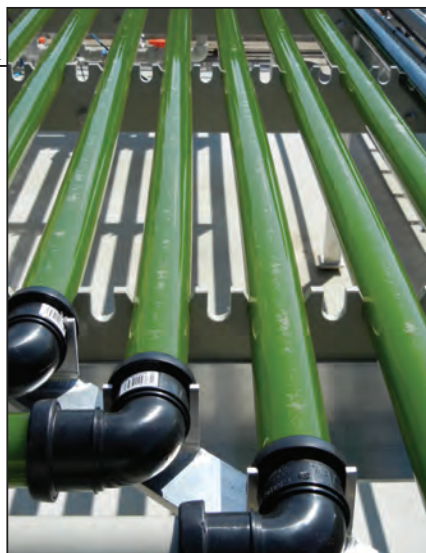
FIGURE 1. Algae flow through the tubes in this horizontal algae reactor
